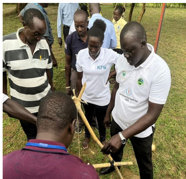
Trainees making the A-frame, a locally made contour tracing for ground levelling equipment. Photo: WFP/Felix Andi
